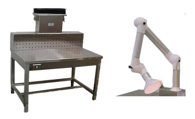
TBJ Backdraft Work Benches are designed to provide an economical vented work bench for controlling odors, gases and chemical fumes by capturing and exhausting air back and away from the work zone of users. The tabletop mounted backdraft plenum is designed to provide an even backdraft capture velocity to efficiently exhaust odors and fumes and provide a healthier, safer work environment.
